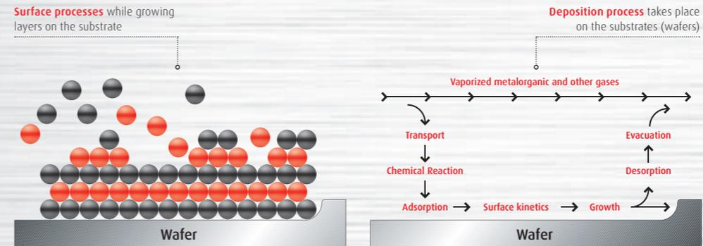
The chemicals used for the deposition process are atoms of group III such as Ga, In, Al, combined with complex organic gas molecules, and atoms of group V such as As, P, N, combined with hydrogen atoms.
