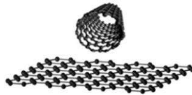
Graphene (2D) and Carbon nanotube (1D) Unique combination of high electrical/thermal conductivity, mobility, flexibility and transparency
