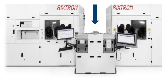
G5+ C dual Planetary reactor module cluster with Cassette-to-Cassette wafer handling
